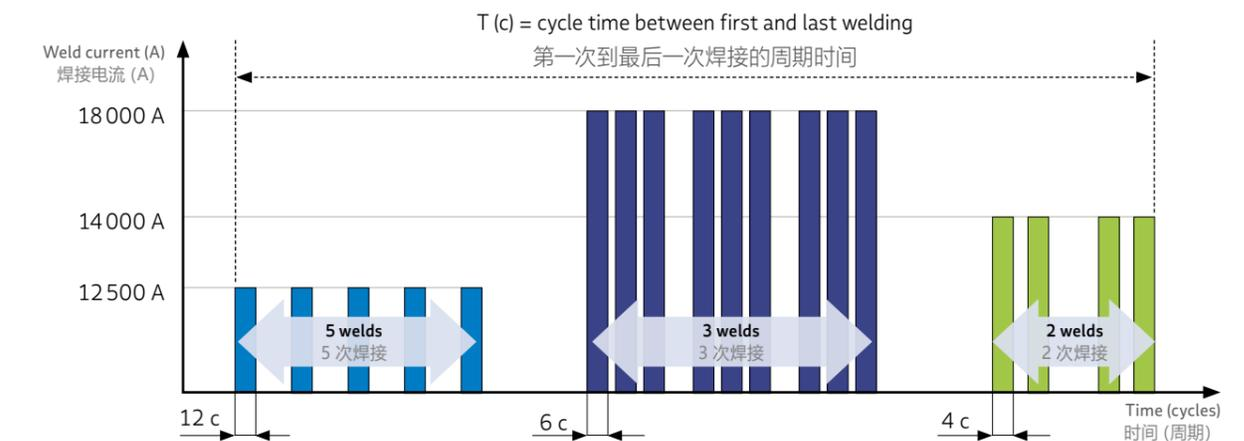
$$I_s = \frac{(5 \text{ welds} \times 12 \text{ c} \times 1 \text{ puls} \times 12500 \text{ A}) + (3 \text{ welds} \times 6 \text{ c} \times 3 \text{ puls} \times 18000 \text{ A}) + (2 \text{ welds} \times 4 \text{ c} \times 1 \text{ puls} \times 14000 \text{ A})}{(5 \text{ 焊接} \times 12 \text{ c} \times 1 \text{ 脉冲}) + (3 \text{ 焊接} \times 6 \text{ c} \times 3 \text{ 脉冲}) + (2 \text{ 焊接} \times 4 \text{ c} \times 1 \text{ 脉冲})}$$
