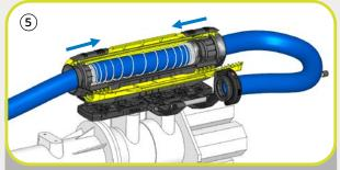
The dresspack is inserted into the LSH Delta. The LSH Delta is closed using the closing latches
