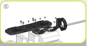
The base plate is installed on the robot. The cable clamp is assembled to the side arm. The side arm / support arms are assembled to the base plate. The aluminum bar is fixed on the arms by tightening the screws.
