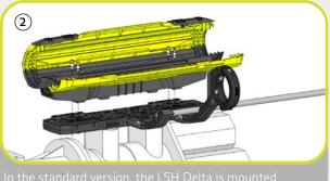
to the base plate with a screw-connection.
