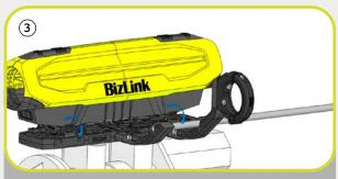
In the premium version, the LSH Delta is slid onto the base plate using the slide & click adapter...
