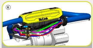
Detailed information for dresspack installation must be considered. During commissioning, ensure that the installation is free of collisions.
