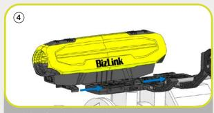
... and then fixed in the desired position using the adapter locks.
