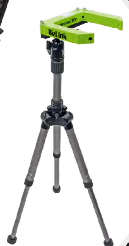
Mobile calibration case for the initial calibration of unknown tools and fixtures (TCP & Base) 用于未知工具和夹具 (TCP 和底座) 初始校准的便携式校准箱
