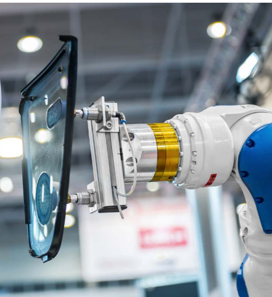
The laser detects features such as curves or edges. 激光检测曲线或边缘等特征。
